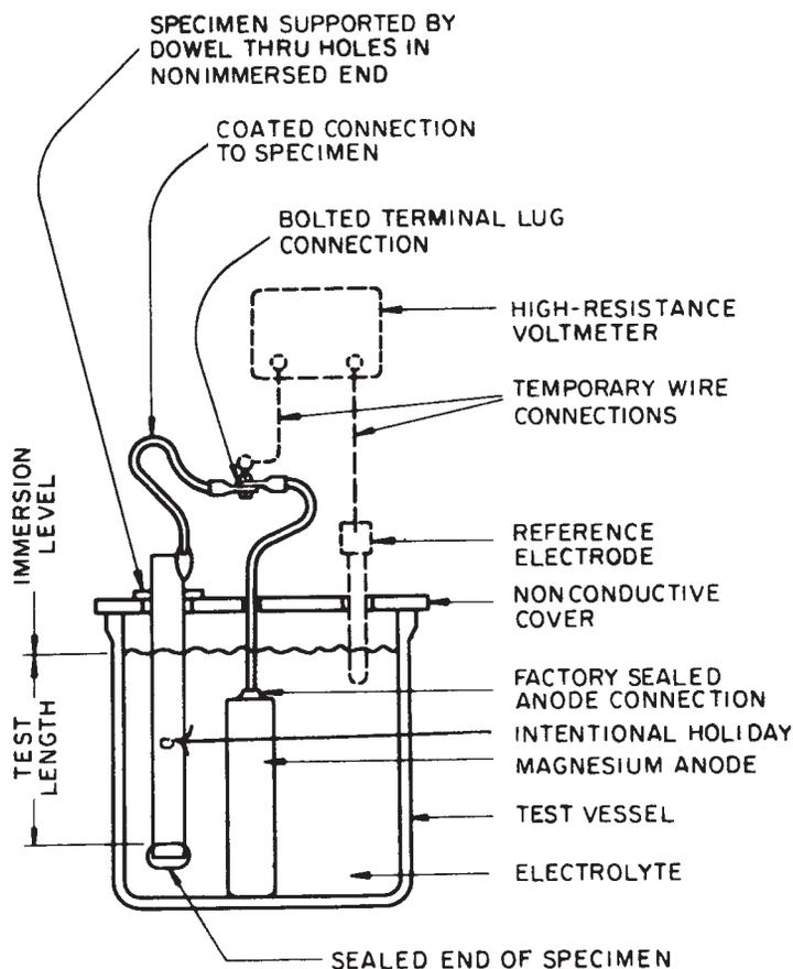
NOTE 1—Test hole made in non-immersed area after testing not shown (see Fig. 5).
